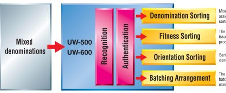
More stackers and larger stacker capacity let you sort by denomination, fitness sorting, and orientation sorting with fewer steps and a shorter overall processing cycle. Increased TWIN reject pocket capacity improves processing time.
